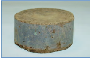
R3 road base has higher compressive strength than asphalt.
